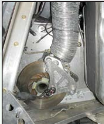
Auxillary brake cooling duct keeps the binders cool.
